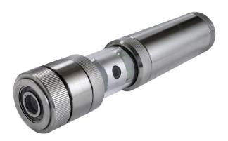
Composed by a downview camera and a 360° free rotating camera for detailed surveys of boreholes and wells. The downview camera provides a perspective image of the borehole. The sideview camera allows the operator to see cracks, damage or other anomalies. The powerful LED engine provides illumination for boreholes up to 600 mm of diameter.
